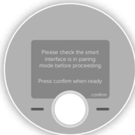
To re-pair go to section E in the Halo Combi installation instructions. You can also find a copy of the installation guide at [www.idealboilers.com](http://www.idealboilers.com)
